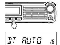
3. Press the [MHz(SETUP)] key momentarily, and then rotate the DIAL knob to select "AUTO".
